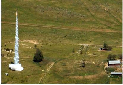
In 2010, the ULA interns upgraded the rocket by using the 2009 Future rocket as the upper stage of the 2010 Future rocket. They built a new booster stage, powered by two clustered N2000W engines. The 2010 Future stood 25 feet tall and weighed 280 lbs. at liftoff. It was the largest rocket ever launched in the state of Colorado!
