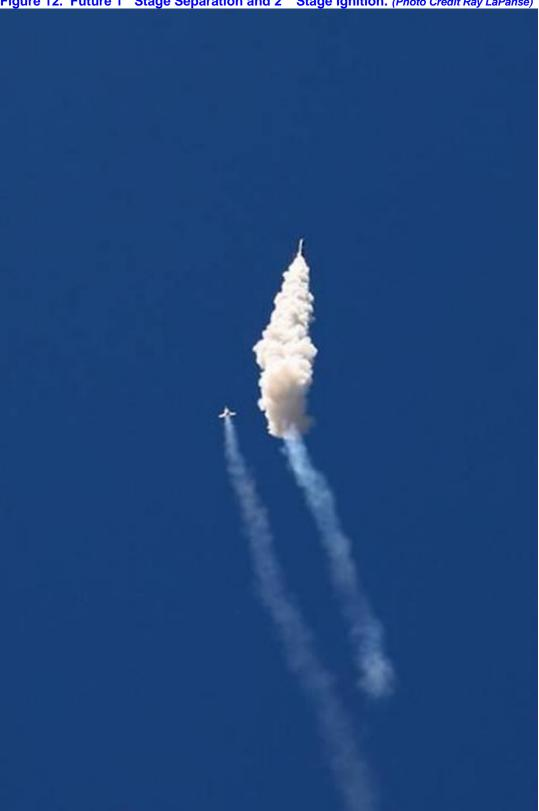
Figure 12. Future 1<sup>st</sup> Stage Separation and 2<sup>nd</sup> Stage Ignition. (Photo Credit Ray LaPanse)
