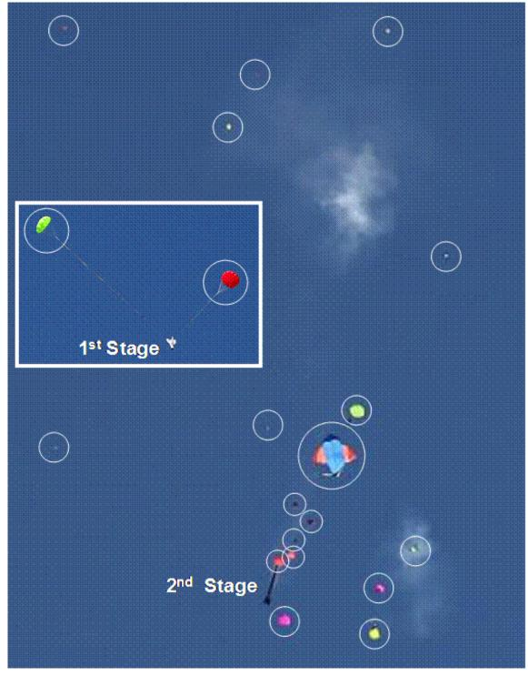
Figure 13. Future Rocket After deployment of its 20 Parachutes - 2 for 1<sup>st</sup> Stage, 6 for 2<sup>nd</sup> Stage, 12 for Payloads *(Photo Credit Ray LaPanse)*
